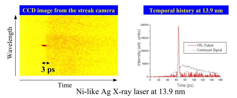
The duration of the XRL pulse at 13.9 nm was measured (after deconvolution) to be  $(1.8 \pm 0.7)$  ps
