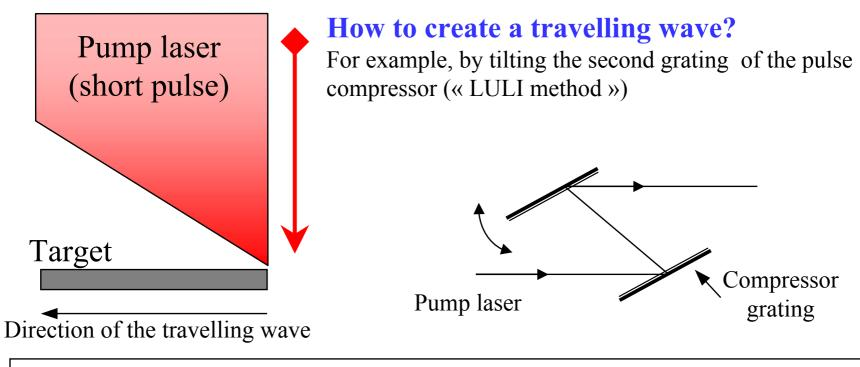
This method allows to control exactly the speed of the travelling wave
