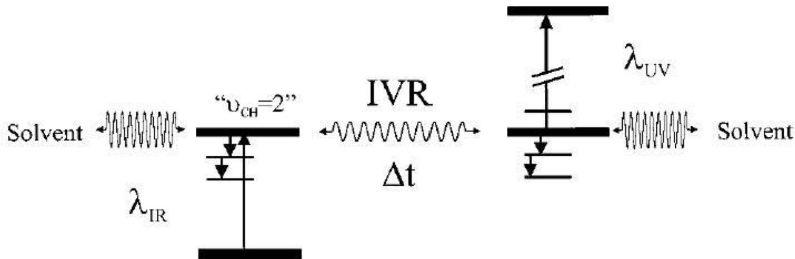
**Figure 1.** Experimental scheme. In our pump-and-probe experiment the first near-IR femtosecond-laser pulse prepares a vibrationally excited molecule with an energy of  $4000\text{--}6000\text{ cm}^{-1}$  in its ground electronic state, and a second laser pulse, tuned to the red wing of the electronic transition in the UV, measures the change in absorption induced by the first laser pulse.
